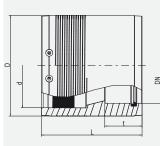
Smooth material transition of HD-PE pipes (SDR 33 - SDR 17) to PVC/PP pipes in house service connections. HD-PE end with integrated coupler. PVC/PP end as slip-on coupler with SBR lip seal and a large insertion depth.
