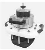
Clamping unit designed for FRIAFIT sewage saddles ASA TL and FRIAFIT transition saddles ASA TL KG, specifically for HDPE Close Fit Inliners DN 200 to DN 500 and for HDPE pipes d 630. For clamping and creating the necessary joining pressure during fusion. Comprising ASATOP clamping unit with toggle anchor, hole saw (Ø 95 mm) with hole saw adapter SDS, centre drill and extension, and compressed air pump. The tool is delivered in a transport box.
