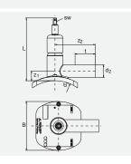
For flexible adaptation to all pipe diameters in indicated range by means of the FRIATOP Clamping device (see application picture and product range FRIATOOLS Ref.-No. 613350). Stainless steel activating spindle 1.4305. No further insulation necessary.
