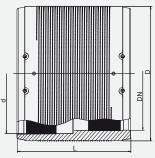
For connection from relining pipe to standard pipe. With exposed heating coils for optimal heat transfer, large insertion depth, wide fusion zone plus cold zones at the end and in the transition area to prevent the flow of molten material for use without holding devices. Gap reduction between coupler and pipe possible through special preheating barcode. For processing refer to relining installation instructions..
