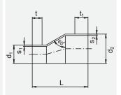
HD-PE long spigot fitting for installation with FRIAFIT electrofusion coupler.
