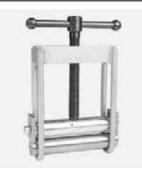
Manual squeeze-off tool for the temporary shutoff of HDPE and PE-Xa pipes d 63 - d 125 in SDR 11 and SDR 17.6.
