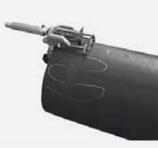
For the reliable removal of the oxide layer of HDPE and PE-Xa pipes. Scraper blade made of carbide with 2 edges (twice the service life). Consistent swarf removal due to spring mounted scraper blade and automatic feed. With quick adjustment of the scraping length and exchangeable clamping slide for the dimensions d 75 - d 225 and d 250 - d 400. The tool is delivered in a transport box.
