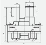
For space saving horizontal installation. Leak free and swarfless tapping up to 10 bar (gas) or 16 bar (water). Integral drill with upper and lower stop, guided in a metal sleeve. With exposed heating element for optimal heat transfer.
