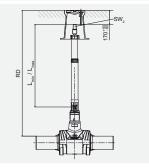
To operate the FRIALOC PE shut-off valve from the surface box. Optimally matched, can be individually extended to the required covering height. With KlickFix coupler for easy installation. Made of galvanised steel or stainless steel
