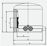
With exposed heating coil for optimal heat transfer, large insertion depth, extra wide fusion zone plus cold zones at the end to prevent the flow of molten material.
