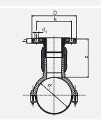
Compact fitting in HD-PE. Manufactured combination of FRIALEN spigot saddle, coupler and FRIALEN Full Faced Flanges EFL (compact flange). Saddle with exposed heating coil for optimum heat transfer. Tapping in pressure free condition or, using an additional shut-off valve, under operating pressure by means of standard tapping equipment (we recommend Hütz & Baumgarten (www.huetz-baumgarten.de)). We recommend steel-reinforced elastomeric gaskets.
