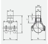
Compact transition fitting. HD-PE-saddle with exposed heating element for optimal heat transfer. Gunmetal adapter permanently anchored in the HD-PE. Cannot be released or rotated. To accept normal commercial brass valves. Metallic materials in contact with drinking water acc. to the recommendation of Umweltbundesamt, Germany.
