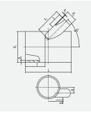
HD-PE long spigot fitting for installation with FRIAFIT electrofusion coupler. Pipe colour black with bright inner surface (according to availability)
