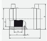
Can also be used as repair couplers. With exposed heating coils for optimal heat transfer, large insertion depth, wide fusion zones plus cold zones at the end and in the middle to prevent the flow of molten material, for use without holding devices.
