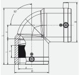
With exposed heating coils for optimal heat transfer, large insertion depth, wide fusion zones plus cold zones at the end and in the middle to prevent the flow of molten material, for use without holding devices.
