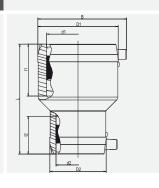
With exposed heating coils for optimal heat transfer, large insertion depth, wide fusion zones plus cold zones at the end and in the middle to prevent the flow of molten material, for use without holding devices.
