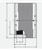
With exposed heating coils for optimal heat transfer, large insertion depth, wide fusion zones plus cold zones at the end and in the middle to prevent the flow of molten material, for use without holding devices.
