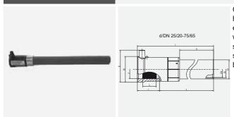
Compact transition fitting. HD-PE end with exposed heating coils for optimal heat transfer, large insertion depth, wide fusion zone plus cold zones at the end and in the transition area to prevent the flow of molten material, for use without holding devices. Steel end permanently anchored in the HD-PE. Self sealing patented sealing geometry without elastomer seal. For use in gas systems. Steel pipe sockets marked by restrutting (for use with gas up to 10 bar).
