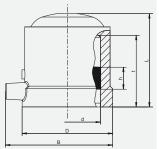
With exposed heating coils for optimal heat transfer, large insertion depth, wide fusion zone plus cold zones at the end to prevent the flow of molten material.
