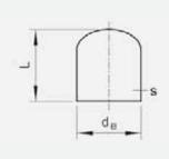
PE 100 Maximum testing pressure 0.5 bar in accordance to DIN EN 1610
