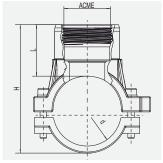
Compact saddle fitting with threated outlet for the jointing of irrigation systems for green fields, e.g. playing fields or golf courses. HD-PE saddle with exposed heating element for optimal heat transfer. Integrated threaded brass sleeve for safe adaption of PVC-ACME fittings.
