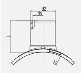
For integration of a branch line in PE pipelines – unpressurised or under operating pressure. Compact fitting made of HD-PE. Saddle with exposed heating element for optimal heat transfer. Outlet spigot for processing with FRIALEN couplers MB or UB. Suitable for all pipe diameters in the given range.
