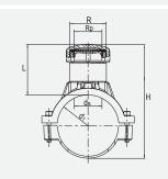
Compact fitting suitable for available balloon shut-off equipment. HD-PE saddle with exposed heating element for optimal heat transfer. Brass-guide thread permanently and immovably anchored in the HD-PE. Cannot be released or rotated. Includes brass plugs with square recess. Protection against access to the stack by fusing on a FRIALEN SPAK (when using d 63 through cap K order no. 612310).
