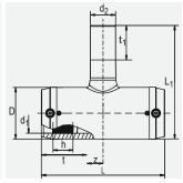
With exposed heating coils for optimal heat transfer, large insertion depth, wide fusion zones plus cold zones at the end and in the middle to prevent the flow of molten material, for use without holding devices. Separate fusion zones. Spigot outlet SDR 11 for processing couplers UB/MB.
