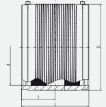
For the jointing of HD-PE pipes in non-pressure and pressure systems for sewage, wastewater or drinking water pipes. With exposed heating coils for optimal heat transfer, large insertion depth, extra wide fusion zones plus cold zones at the end and in the middle to prevent the flow of molten material for use without holding devices. With pin indicator for visually checking fusion.
