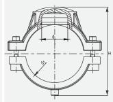
Compact fitting consisting of one repair saddle and one reinforcing saddle for the repair of minor pipe damage. With exposed heating elements for optimal
