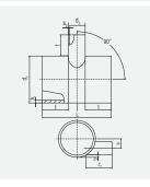
HD-PE long spigot fitting for installation with FRIAFIT electrofusion coupler. Pipe colour black with bright inner surface (according to availability)
