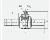
Compact ball valve in HD-PE with spigots for use with FRIALEN couplers MB or UB. No corrosion proofing required. Open and closed position with definite stop. Maintenance free ball valve, operated by a rod (e.g. FRIALEN BS Installation kits for Ball Valves and Tapping Ball Valves). Maximum clearence diameter d<sub>1</sub>.
