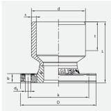
Compact fitting manufactured by factory from HD-PE reducer and FRIALEN EFL Full Face Flanges. Specially suited for the horizontal connection of flange valves to FRIALEN T-pieces T for reduced branches in DN 80 and DN 100. For the vertical connection of hydrants using our elbow including foot support WF 90° d 110 or the T-piece T, the installation depth must be taken into consideration. No internal welding bead at the weld seam of the reduction. Steel-reinforced elastomeric gaskets recommended.
