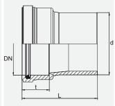
Smooth material transition in domestic range between HD-PE pipes (SDR 33 - SDR 17) and PVC/PP pipes. HD-PE side can be fused with FRIAFIT AM sewage coupler, bends ABM/ABMS or with the outlet of the FRIAFIT ASA TL sewage saddle. PVC/PP side as socket coupler with SBR lip seal gasket and large insertion depth.
