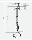
Telescopic actuating rod for operation of the FRIALEN DAV from the street cap. Stepless adjustment in the stated range (RD) without the use of tools, even in the installed state. Self supporting in any extended position. Corrosion proof.
