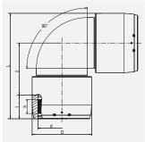
With exposed heating coils for optimal heat transfer, large insertion depth, wide fusion zones plus cold zones at the end and in the middle to prevent the flow of molten material, for use without holding devices. Separate fusion zones. Handling at the construction site is made easy thanks to the fused-on eyebolts.
