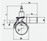
Compact fitting in HD-PE with no threaded connection. Actuating spindle in stainless steel 1.4305. No re-insulating required. Leak free and swarfless tapping up to 10 bar (gas) or 16 bar (water). Integral drill with upper and lower stop, guided in a metal sleeve. Max. 9 turns to activate "OPEN/CLOSF"
