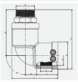
Compact transition fitting. HD-PE end with exposed heating coils for optimal heat transfer, large insertion depth, wide fusion zone plus cold zones at the end and in the transition area to prevent the flow of molten material for use without holding devices. Stainless steel end permanently anchored in the HD-PE. Cannot be released or rotated. Self sealing patented sealing geometry without elastomer seal. For use in water systems.
