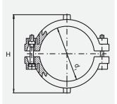
Compact fitting manufactured from 2 HD-PE saddles for the repair of minor pipe damage. With exposed heating elements for optimal heat transfer.
