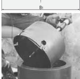
For integration of a branch line or vent in PE pipelines with large diameters – unpressurised or under operating pressure. Compact fitting made of HD-PE. Saddle with exposed heating element for optimal heat transfer. Outlet spigot for processing with FRIALEN couplers MB or UB.
