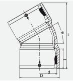
Little space required thanks to compact design as well as angle spacings of 15°, 30°, 45° facilitate a comfortable pipeline routing. Fusion couplers integrated on both ends to reduce the assembly time with exposed heating coils for an optimal heat transfer. The smooth, hydraulically optimised internal contour offers a level passage when pipes SDR 17/17.6 are used. The bright surface facilitates an optimal view during camera inspection. With pin indicator for visually checking fusion
