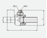
Compact ball valve made from HD-PE with spigots for processing with FRIALEN MB or UB couplers. Full port valve passage in line with internal diameter of pipe socket. No corrosion prevention measures necessary. Open and closed position at defined stop. Maintenance free shut-off valve activated by a rod (e.g. FRIALEN BS Installation kits for Ball Valves and Tapping Ball Valves).
