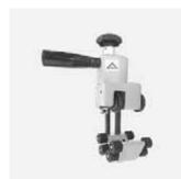
For the reliable removal of the oxide layer of HDPE and PE-Xa pipes. Scraper blade made of carbide designed as reversible blades with 2 cutting edges (twice the service life). Universal scraping ranges, no dimension adjustment required. Even swarf removal thanks to a spring-loaded scraper blade and automatic feed. The tool is delivered in a transport box.
