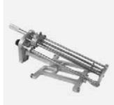
For the reliable removal of the oxide layer of HDPE pipes for half or entire coupler length. Scraper blade made of carbide for a long life. Even swarf removal thanks to a spring-loaded scraper blade and automatic feed. Includes a replacement blade. The tool is delivered in a transport box.
