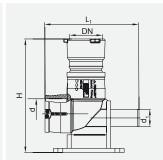
For jointing of hydrant with spigot according to BAIO system as alternative to flange connection. Compact fitting manufactured from FRIALEN 90° elbow with base (see WF 90°) and BAIO coupler made from ductile cast iron including sealing ring. BAIO coupler anchored in PE moulded part. Cannot be released or rotated. Please observe specific processing instructions for "BAIO" system. For below floor hydrants the safety device against dirt and distortion for BAIO spigots is required.
