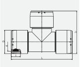
With exposed heating coils for optimal heat transfer on all 3 sides, large insertion depth, wide fusion zones plus cold zones at the end and in the middle to prevent the flow of molten material, for use without holding devices. Separate fusion zones. Handling at the construction site is made easy thanks to the fused-on eyebolts.
