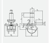
PE 100 SDR 11 Maximum working pressure 16 bar (water)/10 bar (gas)
