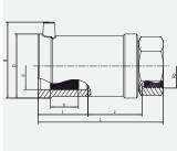
Compact transition fitting. HD-PE end with exposed heating coils for optimal heat transfer, large insertion depth, wide fusion zone plus cold zones at the end and in the transition area to prevent the flow of molten material for use without holding devices. Steel end permanently anchored in the HD-PE. Self sealing patented sealing geometry without elastomer seal. For use in gas systems.
