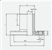
Flange Adaptor and flange as a factory made flange piece. Metal insert in the flange to prevent creep. Spigot end for use with FRIALEN couplers MB or UB. Steel-reinforced elastomeric gaskets recommended. Please observe the bolting torques of the gasket manufacturer.
