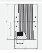
With exposed heating coils for optimal heat transfer, large insertion depth, wide fusion zones plus cold zones at the end and in the middle to prevent the flow of molten material, for use without holding devices.
