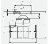
Compact fitting in HD-PE. Factory made combination made from FRIALEN T-Piece, Reducer and Full Faced Flanges (fixed flange). T-Piece with exposed heating coils for optimal heat transfer, large insertion depth, wide fusion zones plus cold zones at the end and in the middle to prevent the flow of molten material for use without holding devices. No internal welding bead at the weld seam. Steel-reinforced elastomeric gaskets recommended. Additional washers are necessary for the flange reducer.
