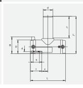
Straight connector with exposed heating coils for optimal heat transfer, large insertion depth, wide fusion zones plus cold zones at the end and in the middle to prevent the flow of molten material, for use without holding devices. Up to and including d63 extra long spigot outlet dimensioned for 2 fusion operations.
