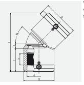
With exposed heating coils for optimal heat transfer, large insertion depth, wide fusion zones plus cold zones at the end and in the middle to prevent the flow of molten material, for use without holding devices.
