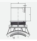
For the connection of fused HD-PE service pipes or side branches to clay or concrete mains. For new installations as well as rehabilitation - without separating or completely exposing the main sewer. The outlet spigot d 160 offers a levelled passage when using pipes SDR17/17.6. Its bright inner surface facilitates an optimal view during camera inspection. Fusible with FRIAFIT coupler AM or FRIAFIT bends ABM/ABMS.
