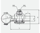
Compact tapping ball valve in HD-PE. Factory made combination of FRIALEN Saddle Moulding and FRIALEN Ball Valve with spigot for space and cost saving horizontal installation especially for integration of branches into mains under operating pressure. Leakage and swarf free tapping up to 10 bar (gas) and standard tapping equipment (we recommend Hütz & Baumgarten (www.huetz-baumgarten.de)). With exposed heating element for optimal heat transfer.
