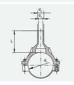
Compact fitting in HD-PE, saddle with exposed heating element for optimal heat transfer and outlet spigot for use with FRIALEN couplers MB or UB. Swarfless tapping in the depressurised state by means of commercial drilling units (we recommend Hütz & Baumgarten (www.huetz-baumgarten.de)).
