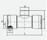
With exposed heating coils for optimal heat transfer, large insertion depth, wide fusion zones plus cold zones at the end and in the middle to prevent the flow of molten material, for use without holding devices. Separate fusion zones. Outlet spigot SDR 11 for processing of UB/MB couplers. Other branch dimensions can be created using MR d 225/160 or MR d 110/90 and MR d 110/63. Handling at the construction site is made easy thanks to the fused-on eyebolts.
