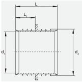
For the repair of water service pipes in the depressurised state. Prevents the ingress of water into the fused area of the FRIALEN MB or UB couplers.
