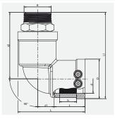
Compact transition fitting. HD-PE end with exposed heating coils for optimal heat transfer, large insertion depth, wide fusion zone plus cold zones at the end and in the transition area to prevent the flow of molten material for use without holding devices. Brass end permanently anchored in the HD-PE. Cannot be released or rotated. Self sealing patented sealing geometry without elastomer seal. For use in water systems. Standard: Brass. Gunmetal on request.
