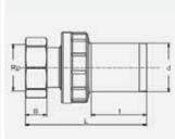
Transition adapter, brass end permanently anchored in HD-PE, with traveling nut for a simple and fast assembling on a fixed male pipe thread. For use in Water area. PE pipe spigot SDR11. Length of the spigot not suitable for FRIALONG couplers.
