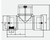
With exposed heating coils for optimal heat transfer on all 3 sides, large insertion depth, wide fusion zones plus cold zones at the end and in the middle to prevent the flow of molten material, for use without holding devices. Straight passage fusible in one-step, therefore a total of only two fusions necessary.
