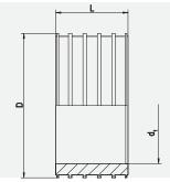
Connecting element between masonry manhole and the FRIAFIT sewage insert sleeve AEM. Anchoring webs (T section) around the entire width for firm and secure fit in manhole with retrospective installation. Defined inner surface for reliable system seal with AEM. Stable inside diameter due to large wall thickness.
