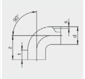
HD-PE long spigot fitting for installation with FRIAFIT electrofusion coupler. Pipe colour black with bright inner surface (according to availability)
