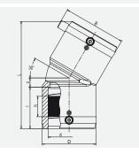
With exposed heating coils for optimal heat transfer, large insertion depth, wide fusion zones plus cold zones at the end and in the middle to prevent the flow of molten material, for use without holding devices.
