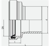
Smooth material transition in domestic range between HD-PE pipes (SDR 33 - SDR 17) and clay pipes (spigot ends). HD-PE side can be fused with FRIAFIT AM sewage coupler, ABM/ABMS bends, or with the outlet of the FRIAFIT ASA TL sewage saddle. Clay side as socket coupler with SBR lip seal gasket and large insertion depth.
