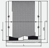
For connection from relining pipe to standard pipe. With exposed heating coils for optimal heat transfer, large insertion depth, wide fusion zone plus cold zones at the end and in the transition area to prevent the flow of molten material for use without holding devices. Gap reduction between coupler and pipe possible through special preheating barcode. For processing refer to relining installation instructions.
