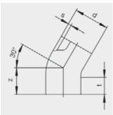
HD-PE long spigot fitting for installation with FRIAFIT electrofusion coupler. Pipe colour black with bright inner surface (according to availability).
