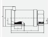
Compact transition fitting. HD-PE end with exposed heating coils for optimal heat transfer, large insertion depth, wide fusion zone plus cold zones at the end and in the transition area to prevent the flow of molten material for use without holding devices. Gunmetal end permanently anchored in the HD-PE. Cannot be released or rotated. Self sealing patented sealing geometry without elastomer seal. For use in water systems.
