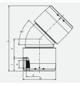
With exposed heating coils for optimal heat transfer, large insertion depth, wide fusion zones plus cold zones at the end and in the middle to prevent the flow of molten material, for use without holding devices. Separate fusion zones. Handling at the construction site is made easy thanks to the fused-on lifting eyes.
