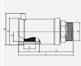
Compact transition fitting. HD-PE end with exposed heating coils for optimal heat transfer, large insertion depth, wide fusion zone plus cold zones at the end and in the transition area to prevent the flow of molten material for use without holding devices. Steel end permanently anchored in the HD-PE. Self sealing patented sealing geometry without elastomer seal. For use in gas systems.
