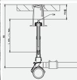
New telescopic actuating rod DBS (EBS) for operation of the new DAV from the street cap. Stepless adjustment in the stated range (RD) without the use of tools, even in the installed state. Self supporting in any extended position.
