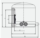
With exposed heating coil for optimal heat transfer, large insertion depth, wide fusion zone plus cold zones at the end to prevent the flow of molten material, for use without holding devices.
