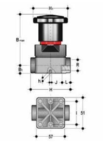
**CMFF**Compact diaphragm valve with BSP threaded female ends
